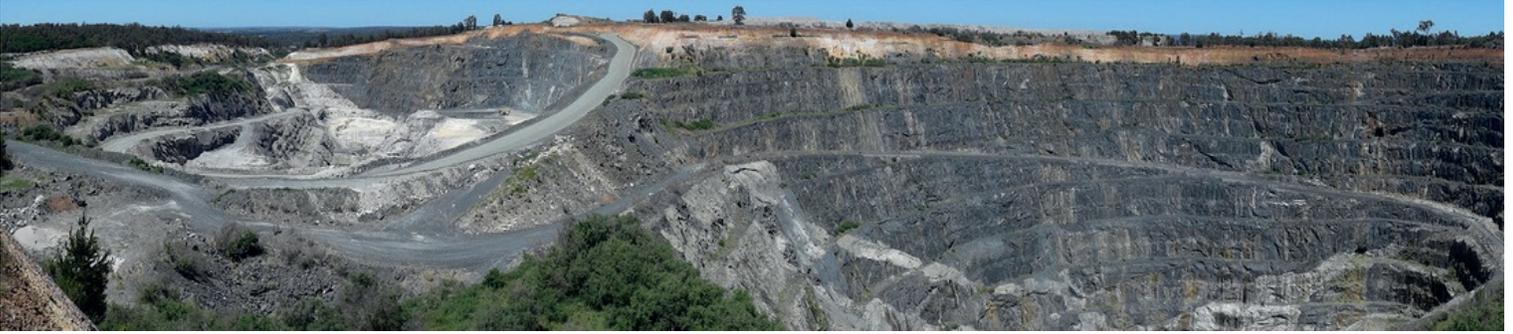
Pictures on this page: [The Greenbushes Mine](#) in Western Australia, jointly owned by US-based Rockwood/Albemarle and China's Sichuan Tianqi Lithium Industries (sources: click on pictures). The pegmatite deposit intrudes along a major northwest regional fault zone. It is approximately 2,525 million years old. The pegmatite consists of a large main zone over 3 km long and up to 300 m wide with numerous smaller pegmatite dikes and pods flanking the main body.
